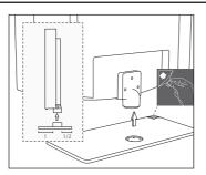
Peel off the protective plastic cover then attach the stand base to the stand neck.
