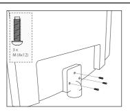
Attach the stand neck to the rear of the TV set using the 3 x M(4x12)
